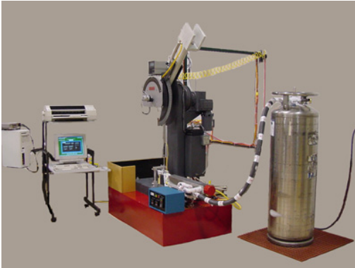
MPM In-situ Heating & Cooling - Large Capacity Machine Installation (U-Hammer)
