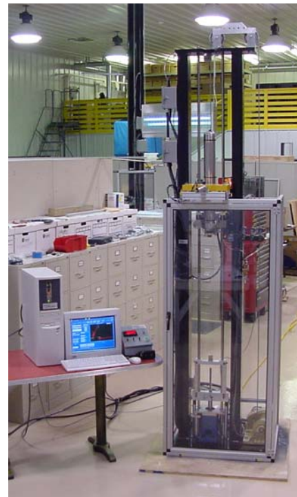
MPM drop tower test machine configured for ASTM D 3763 plastic puncture test
